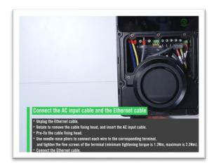
Use needle-nose pliers to connect each wire to the corresponding terminal
