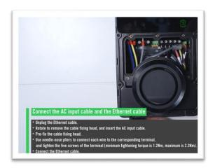
6. Connect all wire to the corresponding terminal and Ethernet cable
